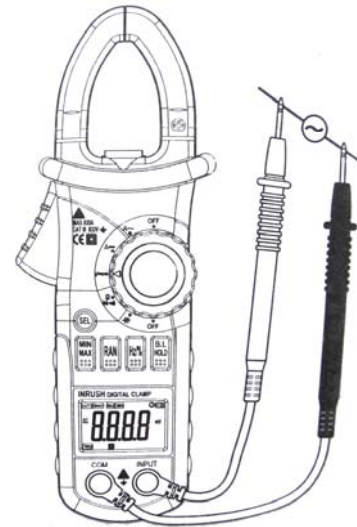
Figure 6. Measuring AC Voltage
